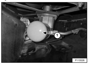
Put a suitable container below the filter, remove the filter (Item 1) [Figure 250], and clean the filter base.
