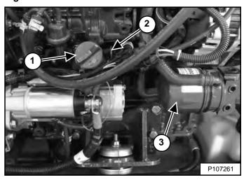
Open the rear door, remove the oil filter (Item 3) [Figure 213], and clean the filter base.
