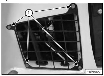
Remove the right side access cover bolts (Item 1) [Figure 241] and remove the access cover. (Lift arms shown raised for visual clarity.)
