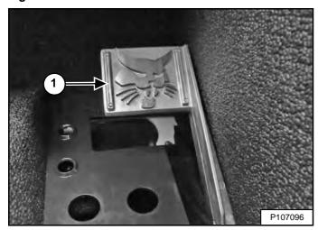
SJC equipped machines have a foot operated engine speed control pedal (Item 1) **[Figure 38]** in addition to the engine speed control lever. The pedal is located on the right side floor above the footrest.
