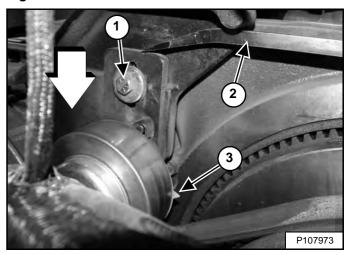
Loosen the spring loaded drive idler mounting bolt (Item 1) [Figure 284].
