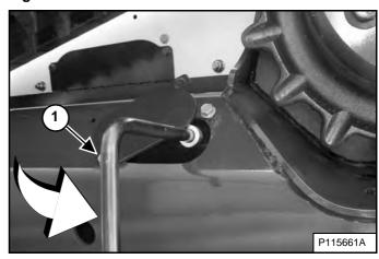
Tighten the access cover bolt (Item 1) [Figure 273] to secure the tool.
