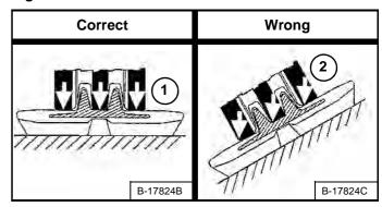
The track carriage components will wear faster when operated on a slope. When the machine is operated on a level surface, the weight of the machine is distributed throughout the entire surface of the rollers to the tracks (Item 1). When operated on a slope, the weight is directed to the edge of the rollers and against the lugs of the track (Item 2) **[Figure 152]** which causes increased wear.
