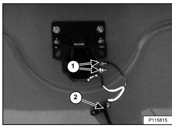
Inspect the back-up alarm electrical connections (Item 1) [Figure 175], wire harness (Item 2) [Figure 175], and back-up alarm switches (if equipped) (Item 1) [Figure 176] for tightness and damage. Repair or replace any damaged components.
