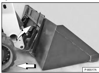
Tilt the Bob-Tach forward and drive the loader backward, away from the bucket or attachment [Figure 140].
