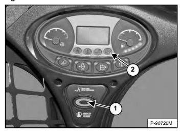
(Functions Only When The Seat Bar Is Raised And The Engine Is Running) There is a TRACTION LOCK OVERRIDE button (Item 1) [Figure 36] on the left instrument panel that will allow you to use the steering controls to move the loader forward and backward when using the backhoe attachment.
