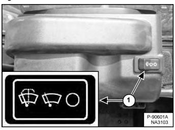
Press the left side of the switch (Item 1) **[Figure 28]** to start the front wiper (press and hold for washer fluid). Press the right side of the switch to stop the wiper.
