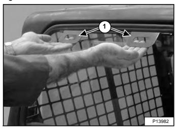
Pull both handles (Item 1) [Figure 47] up and out to remove the rear window.
