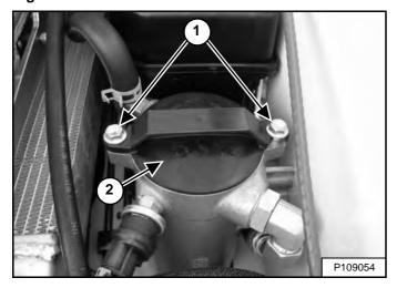
Loosen the bolts (Item 1) and rotate the filter cap (Item 2) [Figure 244] anticlockwise until the cap clears the bolts.
