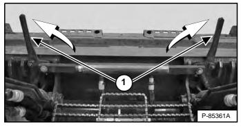
Push and hold BOB-TACH WEDGES "UP" switch (Right Switch Panel) [Figure 141] until levers (Item 1) [Figure 142] are fully raised (wedges fully raised).
