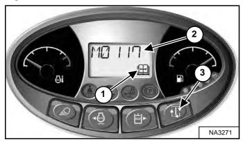
Replace the air filters only when necessary. The service indicator (Item 1) will FLASH. Press the Information button (Item 3) until the display screen shows the service codes. Service code [M0117] (Air Filter Plugged) will show in the display screen (Item 2) [Figure 199] when air filter replacement is necessary.
