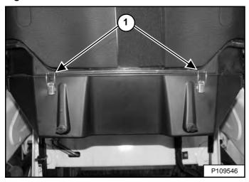
1. Hold the cover in place and fasten two latches (Item 1) [Figure 196].
