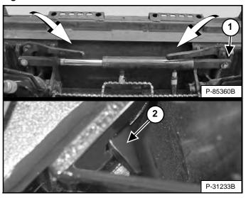
Push and <u>hold</u> BOB-TACH WEDGES "DOWN" switch (Right Switch Panel) [Figure 146] until levers are fully engaged in the locked position [Figure 147] (wedges fully extended through the attachment mounting frame holes).
