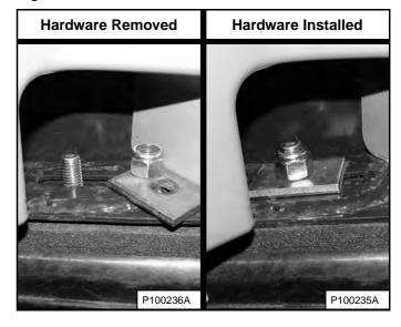
Install the washers and nuts (both sides) [Figure 184].
