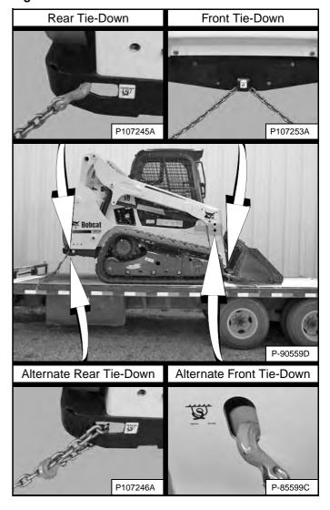
Use the following procedure to fasten the Bobcat loader to the transport vehicle to prevent the loader from moving during sudden stops, or when going up or down slopes **[Figure 163]**.
