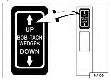
Push and <u>hold</u> BOB-TACH WEDGES "UP" switch (Right Switch Panel) **[Figure 148]** until levers are fully raised (wedges fully raised).
