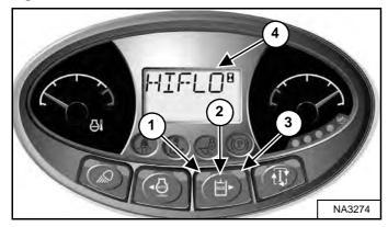
Press the Auxiliary Hydraulics button (Item 2) once to activate the auxiliary hydraulics. The light (Item 1) [Figure 94] is ON.
