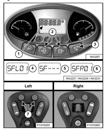
Press the Information button (Item 3) to cycle the data display until the steering drift compensation menu is displayed. The current steering drift compensation setting will appear in the data display (Item 1) [Figure 71].
