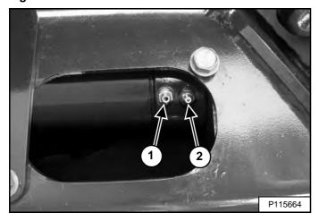
Loosen the access cover bolts and pivot the access cover open [Figure 268].
