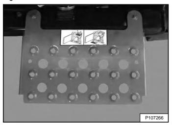
A maintenance platform [Figure 214] is available from your Bobcat dealer to facilitate access when cleaning the engine cooling system.
