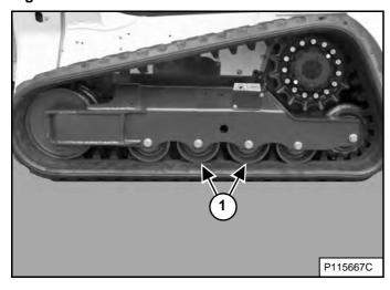
Raise one side of the loader and put jackstands at the front and rear of the loader frame so that the track is about 76 mm (3 in) off the ground [Figure 256]. Lower the loader to the jackstands. Be sure the jackstands do not touch the tracks.
