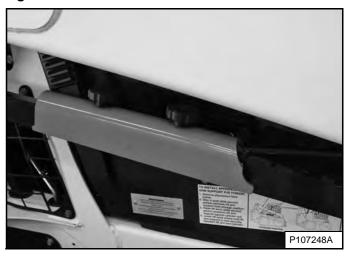
Return the lift arm support device to the storage position and secure with clamping knobs [Figure 173].
