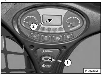
Press the PRESS TO OPERATE LOADER button (Item 1) **[Figure 128]** to activate the BICS<sup>™</sup> and to perform hydraulic and loader functions.
