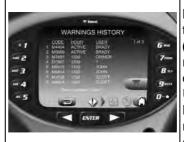
The WARNINGS HISTORY screen will list the Service Code Number (CODE), Hourmeter reading when the error occurred (HOUR), and the User (USER) who was logged in to operate the machine when the error occurred.
