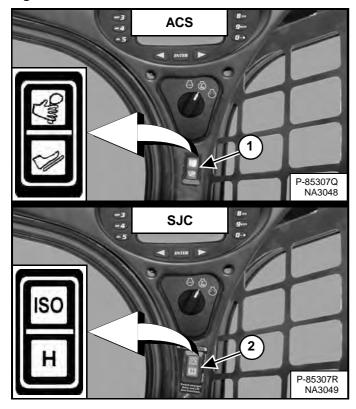
(ACS) Select hand control or foot pedal operation (Item 1) [Figure 127] if equipped with ACS.
