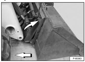
Tilt the Bob-Tach forward and drive the loader backward, away from the bucket or attachment [Figure 149].
