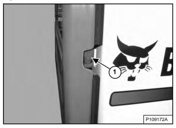
Reach into the slot on the right side of the rear door and pull the latch handle (Item 1) **[Figure 185]**. Pull the rear door open.
