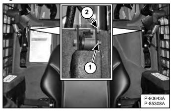
Use compressed air to clean any debris or dirt from the pivot parts. Do not lubricate. Inspect all mounting hardware. The correct hinge nut (both sides) (Item 1) torque is 34 - 38 N•m (25 - 28 ft-lb). The seat bar sensor nut (left side only) (Item 2) [Figure 166] torque is 6 - 8 N•m (50 - 70 in-lb).
