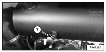
Remove the plug (Item 1) [Figure 252] from the muffler.
