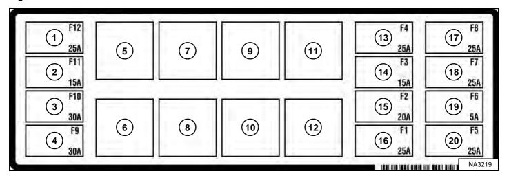
Fuse location and amperage ratings are shown in the table below and on the decal [Figure 231]. Relays are identified by the letter "R" in the AMP column.
