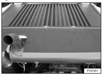
Lift and pull the rear grille backward to remove from the loader [Figure 188].
