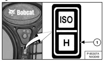
Select the 'H' control pattern by pressing the bottom of the switch (Item 1) [Figure 59].
