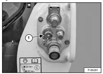
Connect the attachment electrical harness to the attachment control device (Item 1) [Figure 99].
