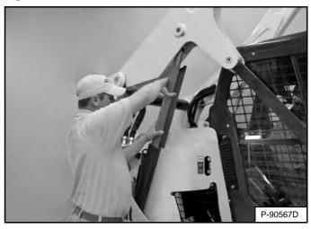
Have a second person install the lift arm support device over the rod of one of the lift cylinders [Figure 170].
