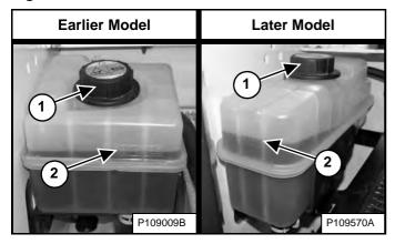
Remove the coolant fill cap (Item 1) [Figure 225].
