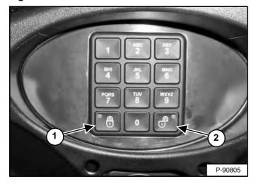
Press and hold the lock (Item 1) and unlock (Item 2) [Figure 313] keys for 2 seconds.
