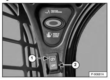
Press the top of the switch (Item 1) **[Figure 35]** to engage the parking brake. The red light in the switch will turn on. The traction drive system is locked.
