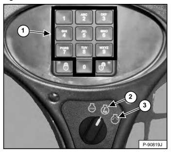
Turn the key switch to RUN (Item 2) **[Figure 120]**. The indicator lights on the left instrument panel will come ON briefly and the instrument panel / monitoring system will perform a self test.
