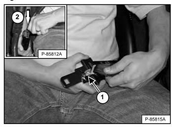
Connect the shoulder belt to the lap belt (Item 1). Pull the lap belt across to the right side of the seat and fasten (Item 2) [Figure 111].
