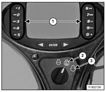
Turn the key switch to RUN (Item 2) **[Figure 125]**. The indicator lights on the left instrument panel will come ON briefly and the instrument panel / monitoring system will perform a self test.
