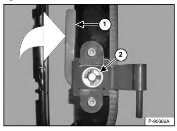
Install cast washers (Item 2) on door hinges taking care to match rectangular surfaces. Hold cast washer firmly against door and rotate latch (Item 1) [Figure 52] up to lock cast washer into position. (Bottom hinge shown.) (Plastic cap shown removed for visual clarity.)
