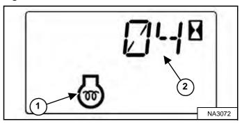
The machine will cycle the glow plugs automatically based on temperature. The engine preheat icon (Item 1) and the cycle time remaining (Item 2) [Figure 126] are displayed in the data display.
