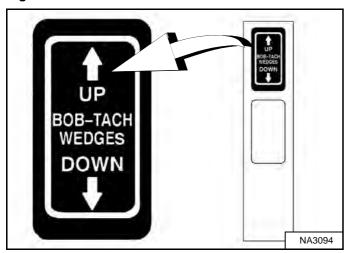
Push and <u>hold</u> BOB-TACH WEDGES "UP" switch (Right Switch Panel) **[Figure 145]** to make sure the levers are fully raised (wedges fully raised).
