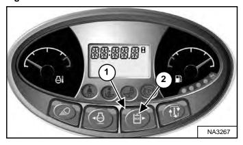
Press the Auxiliary Hydraulics button (Item 2) [Figure 85] once to activate the auxiliary hydraulics.
