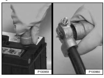
Always clean the battery terminals and cable ends when installing a new or used battery [Figure 235].
