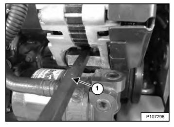
Use a prybar (Item 1) **[Figure 278]** to move the alternator until the belt has 8 mm (0.32 in) movement at the middle of the belt span with 66 N (15 lb) of force.
