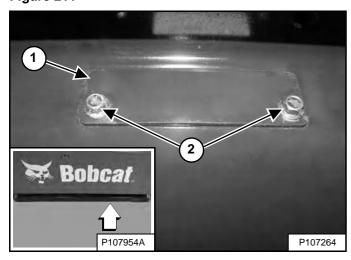
The oil drain hose is located behind a cover (Item 1) under the rear of the loader (Inset) [Figure 211].
