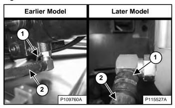
Remove the clamp (Item 1). Pinch off the hose (Item 2) **[Figure 242]** near the fitting and disconnect hose from the fitting. Route the hose out the side of the loader and drain the fluid into a container.
