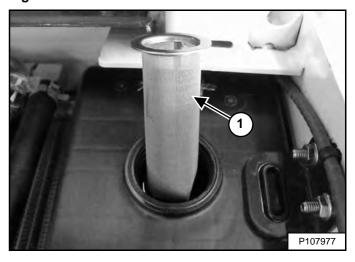
Remove and clean the hydraulic fill screen (Item 1) [Figure 243]. Use low air pressure to dry the screen.
