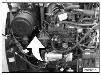
The spring loaded drive idler is located below the air cleaner [Figure 282].
