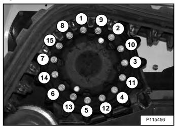
Check the torque of the fifteen track sprocket bolts (Items 1-15) **[Figure 276]**. Use an alternating tightening sequence and then repeat to tighten the bolts to  $127-138 \text{ N} \cdot \text{m}$  (94 -102 ft-lb) torque.
