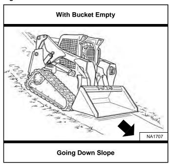
With an empty bucket, go up or down the slope with the heavy end toward the top of the slope [Figure 157] and [Figure 158].
