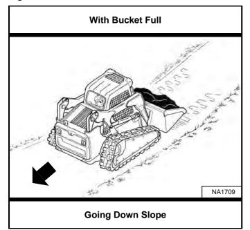
With a full bucket, go up or down the slope with the heavy end toward the top of the slope [Figure 155] and [Figure 156].
