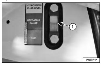
Check the fluid level in the sight gauge (Item 1) [Figure 236]. Keep the fluid level within the operating range.
