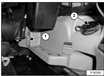
The washer fluid tank is located to the left of the operator seat. Check the fluid level in the sight gauge (Item 1). Remove the cap (Item 2) [Figure 29] to add washer fluid.
