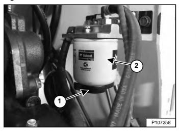
Loosen the drain (Item 1) [Figure 206] at the bottom of the filter to remove trapped water from the filter.
