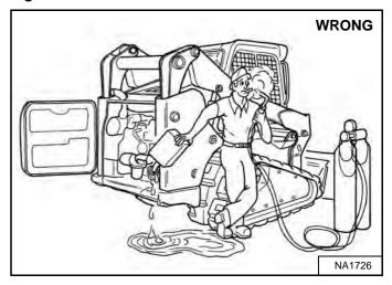
Use a clean, approved safety container to add fuel of the correct specification. Add fuel only in an area that has free movement of air and no open flames or sparks. NO SMOKING [Figure 205].
