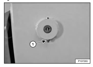
All lift arm and cylinder pivots have a large pin held in position with a retainer bolt and locknut (Item 1) [Figure 303].
