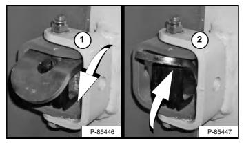
Move the door stop into the engaged position (Item 1) to hold the door open. Move the door stop up (Item 2) **[Figure 186]** to allow the door to close.
