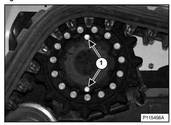
Park the loader so that the plugs (Item 1) [Figure 274] in the hydrostatic drive motor are at the top and the bottom.
