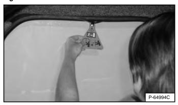
Pull on the tag on the top of the rear window to remove the rubber cord [Figure 43].
