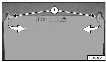
Turn both latches (Item 1) [Figure 41] in until they disengage from the window frame.
