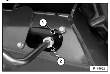
Install the bleed tool (6675936) on the bleed fitting (Item 1), adjust and tighten the collar (Item 2) **[Figure 269]** to fit behind the edge of the access cover.
