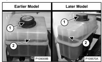
Coolant must be between the top and bottom level markers (Item 2) [Figure 224] when the engine is cold.
