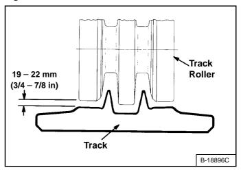
DO NOT put your fingers into the pinch points between the track and the roller. Use a 19 - 22 mm (3/4 - 7/8 in) bolt, dowel or block to check the gap [Figure 266] and [Figure 267].
