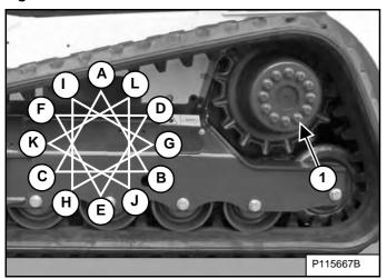
Check the torque of the 12 track sprocket bolts (Item 1) [Figure 275].
