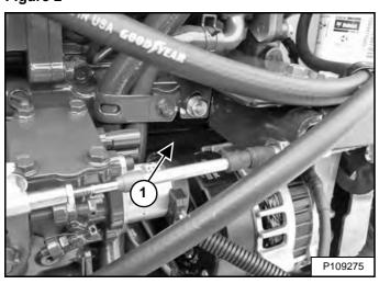
The engine serial number (Item 1) **[Figure 2]** is located on the side of the engine behind the alternator.
