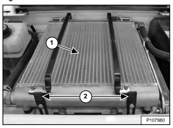
Use low air pressure or water pressure to clean the top of the hydraulic fluid cooler (Item 1) [Figure 218].
