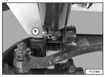
9. Rod End Tilt Cylinder (Both Sides) (2) [Figure 300].
