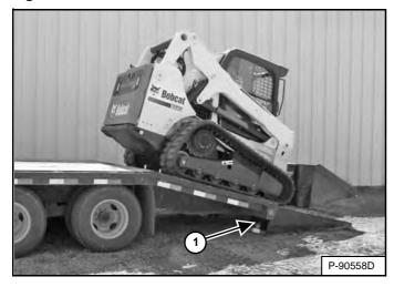
A loader with an empty bucket or no attachment must be loaded backward onto the transport vehicle [Figure 162].
