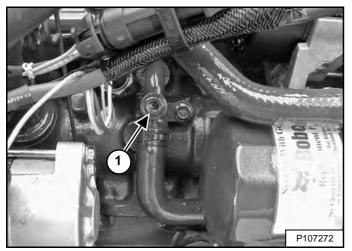
Remove the coolant drain plug (Item 1) [Figure 226] located to the left of the oil filter. Drain the coolant into a container. Install and tighten the plug.
