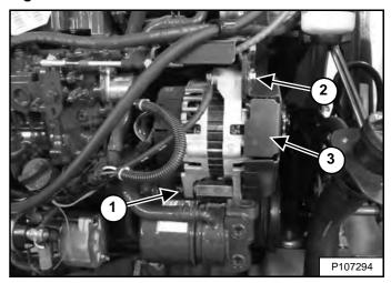
Loosen the bottom alternator mounting nut (Item 1) and remove the top alternator adjusting bolt (Item 2) [Figure 279].
