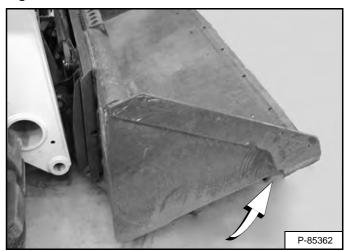
Tilt the Bob-Tach backward until the cutting edge of the bucket (or other attachment) is slightly off the ground [Figure 144]. This procedure will cause the bucket mounting frame to fit up against the front of the Bob-Tach.
