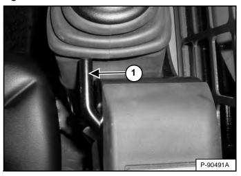
Pull the joystick adjustment levers (Item 1) [Figure 113] up to slide the loader joysticks forward or backward to adjust for comfortable operation. (Right side shown.)
