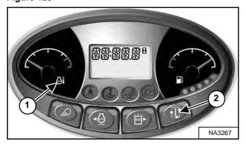
Frequently monitor the temperature and fuel gauges and BICS<sup>TM</sup> lights (all BICS<sup>TM</sup> lights must be OFF to operate loader) [Figure 129].
