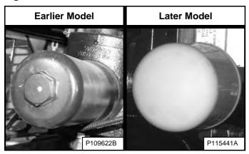
Earlier models use a separate filter housing and filter element. Later models use a spin-on filter [Figure 247].
