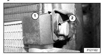
Ensure the air conditioning condenser is installed into the two slotted brackets [Figure 222]. (Right side shown.)
