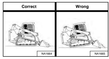
**Digging And Levelling:** Keep the full length of the tracks in contact with the ground [Figure 151] for best traction.
