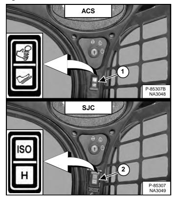
(ACS) Select hand control or foot pedal operation (Item 1) [Figure 117] if equipped with ACS.
