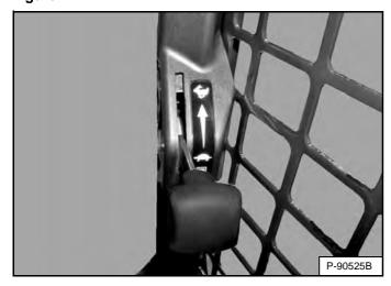
Set the engine speed control to the low idle position [Figure 124].
