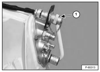
You will need the 14-Pin Attachment Control Device kit (Item 1) **[Figure 100]** to operate early model attachments. See your Bobcat loader dealer.
