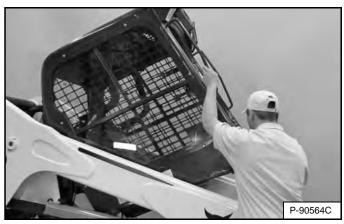
Lift on the grab handles and bottom of the operator cab [Figure 182] slowly until the operator cab is all the way up and the latching mechanism engages.
