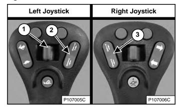
Additional switches (Items 1, 2, and 3) [Figure 101] or [Figure 102] are used to control some attachment functions through the attachment control device.
