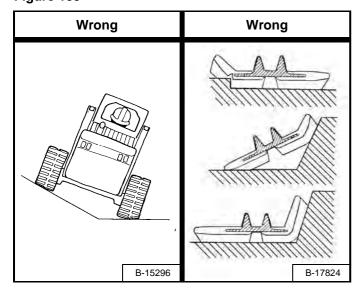
**Operating Conditions:** Avoid operating the loader with one track on a slope and the other on flat ground or with the end of the track turned up against a curb or mound **[Figure 153]**. This can cause the tracks to derail, cracks in the edge of the tracks, or cracks at the edges of the embedded metal.
