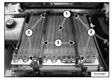
Use low air pressure or water pressure to clean the top of the air conditioning condenser (Item 1) [Figure 216].
