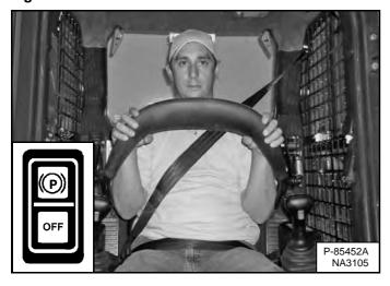
Lower the seat bar and engage the parking brake [Figure 112].
