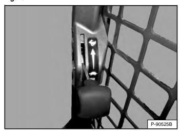
Set the engine speed control to the low idle position [Figure 114].
