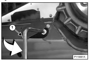
Tighten the access cover bolt (Item 1) [Figure 264] to secure the tool.
