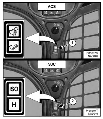
(ACS) Select hand control or foot pedal operation (Item 1) [Figure 122] if equipped with ACS.
