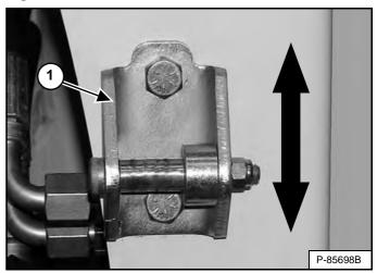
The door latch striker (Item 1) **[Figure 187]** can be adjusted up or down for alignment with the door latch.
