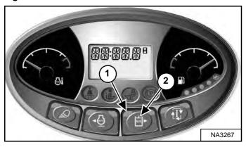
Press the Auxiliary Hydraulics button (Item 2) [Figure 90] once to activate the auxiliary hydraulics.
