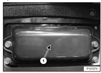
The electrical system is protected from overload by fuses located under the fuse panel cover (Item 1) [Figure 229].
