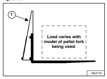
The maximum load to be carried when using a pallet fork is shown on a decal located on the pallet fork frame (Item 1) [Figure 134].
