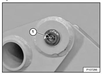
1. Lift Arm Pivot Pin (Both Sides) (2) [Figure 292].
