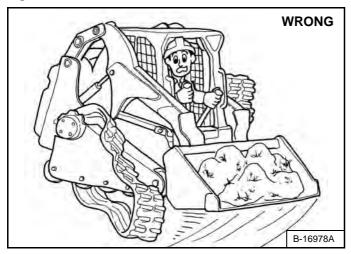
**Turning:** Use a gradual turn (one lever farther forward than the other) instead of a fast turn (one lever forward and one lever backward) on asphalt or concrete surfaces to prevent reduced track life or derailing of tracks **[Figure 150]**.
