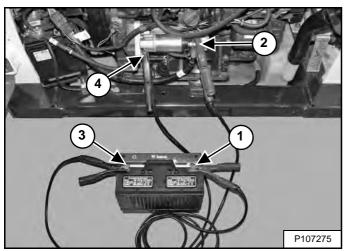
Connect the end of the first cable (Item 1) to the positive (+) terminal of the booster battery. Connect the other end of the same cable (Item 2) **[Figure 233]** to the positive (+) terminal on the engine starter.
