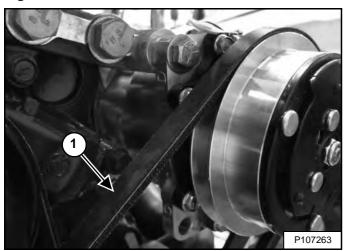
Move the air conditioning compressor until the belt (Item 1) **[Figure 281]** has 4 mm (0.16 in) movement at the middle of the belt span with 17 N (3.8 lb) of force.
