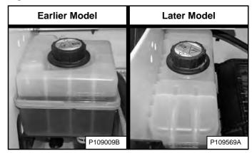
Earlier models have a square coolant tank. Later models have a rectangular coolant tank [Figure 215].
