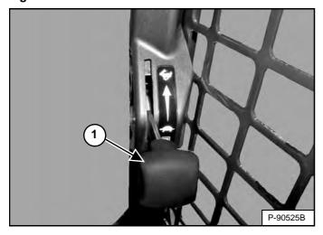
The engine speed control (Item 1) [Figure 37] is located alongside the door frame below the right panel.
