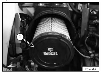
Remove the outer filter (Item 1) [Figure 201] and discard.
