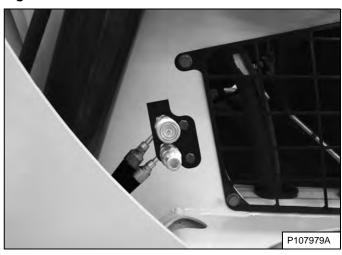
Move the Rear Auxiliary Hydraulic switch (Item 1) [Figure 91] or [Figure 92] to the right or left to change direction of the auxiliary hydraulic fluid flow to the rear quick couplers [Figure 93]. (EXAMPLE: Raise and lower rear stabilisers.) Release the switch to stop fluid flow.
