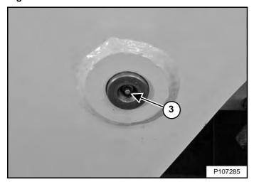
3. Base End Lift Cylinder (Both Sides) (2) [Figure 294].
