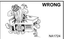
Do not use loader in atmosphere with explosive dust, explosive gas, or where exhaust can contact flammable material.
