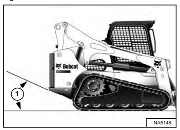
NOTE: The loader should be lifted as close to horizontal as possible, but at no time should the angle of the suspended loader exceed the departure angle (Item 1) [Figure 160] provided in the specifications section. (See Machine Dimensions on Page 198.)
