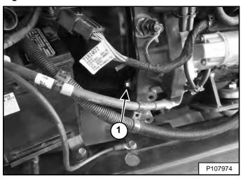
Remove the drive belt shield bolt (Item 1) [Figure 285].
