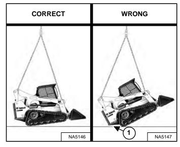
Attach cables or chains to lift eyes [Figure 161].
