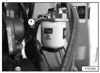
Open the air vent plug (Item 1) [Figure 207] on the fuel filter base.
