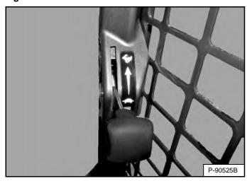
Set the engine speed control to the low idle position [Figure 130].
