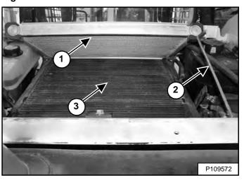
Raise the air conditioning condenser (Item 1) and rotate the support bar (Item 2) into position. Use low air pressure or water pressure to clean the top of the hydraulic fluid cooler and radiator assembly (Item 3) [Figure 221].
