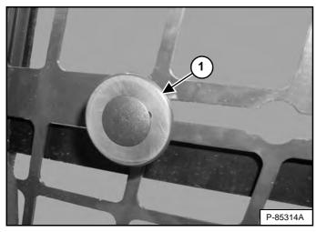
Pull the knob (Item 1) **[Figure 25]** and slide backward to open window. Release knob at cutout to lock in desired position. Pull the knob and slide forward to close window.
