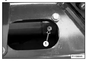
Loosen the access cover bolts and pivot the access cover open [Figure 262].
