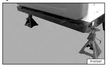
Install jackstands under the rear of the loader frame [Figure 180].
