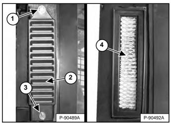
The fresh air filters are located behind the side windows outside the operator cab. (Right side shown) Remove the retaining screw (Item 3) and the filter cover (Item 2) [Figure 190]. (Lift arms shown raised for visual clarity.)
