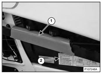
The lift arm support device (Item 1) [Figure 168] is used to support the lift arms while working on a machine with the lift arms up.
