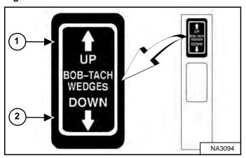
Push and hold the BOB-TACH WEDGES "UP" switch (Item 1) until wedges are fully raised. Push and hold the BOB-TACH WEDGES "DOWN" switch (Item 2) [Figure 307] until the wedges are fully down.
