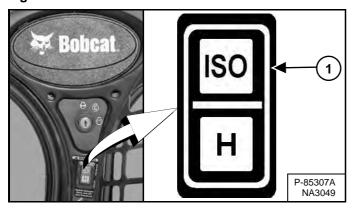
Select the 'ISO' control pattern by pressing the top of the switch (Item 1) [Figure 56].
