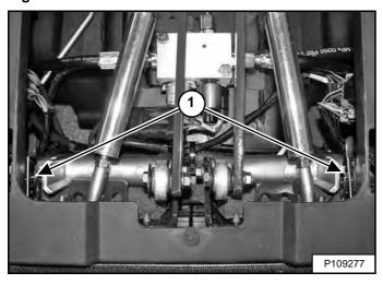
The back-up alarm switches (Item 1) [Figure 176] are located alongside the steering bellcranks. Both switches must be adjusted properly for the back-up alarm to operate correctly.
