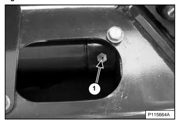
Loosen the access cover bolts and pivot the access cover open [Figure 271].
