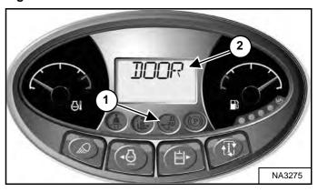
The LIFT AND TILT VALVE light (Item 1) **[Figure 179]** is OFF when the door is <u>closed</u>, the key switch is turned to RUN, the seat bar is lowered, and the PRESS TO OPERATE LOADER button is pressed.
