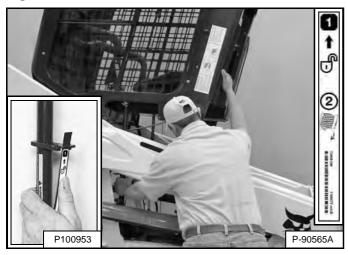
Pull down on the bottom of the operator cab until stopped by the latching mechanism [Figure 183].
