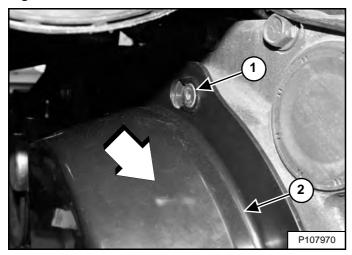
Do **NOT** loosen the drive belt shield mounting bolts (top bolt shown) (Item 1). Slide the drive belt shield (Item 2) **[Figure 286]** toward the back of the loader to unseat the shield from the top and bottom drive belt shield mounting bolts.
