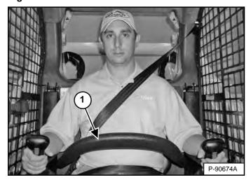
The seat bar restraint system has a pivoting seat bar with armrests (Item 1) [Figure 165].
