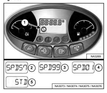
The Speed Management icon (Item 1) [Figure 66] will appear in the display and remain on until the Speed Management button is pressed again or the machine is turned off.
