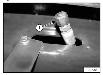
Remove the oil drain cap (Item 1) **[Figure 212]** from the oil drain hose and drain the oil into a container. Recycle or dispose of used oil in an environmentally safe manner.
