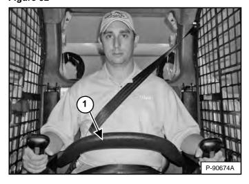
The Bobcat Interlock Control System (BICS<sup>™</sup>) has a pivoting seat bar with armrests (Item 1) [Figure 32]. The operator controls the use of the seat bar.
