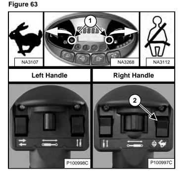
Press the top of the switch (Item 2) on the right handle for high range. The two-speed and shoulder belt icons located on the left instrument panel (Item 1) [Figure 63] will come on.
