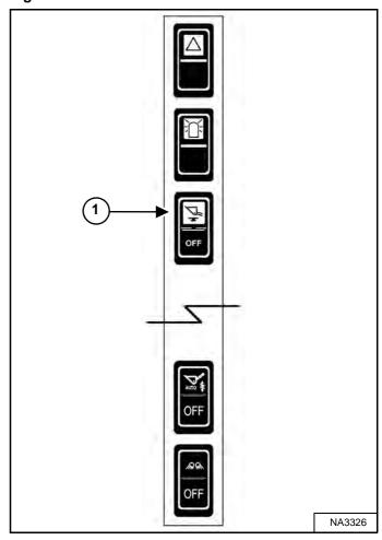
Press the top of the Bucket Positioning switch (Item 1) **[Figure 82]** on the left switch panel to engage the bucket positioning function. The amber light in the switch will turn on. Press the bottom of the switch to disengage. The amber light will turn off.
