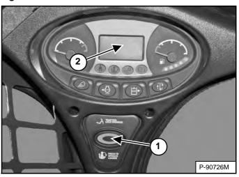
Press the PRESS TO OPERATE LOADER button (Item 1) **[Figure 123]** to activate the BICS<sup>™</sup> and to perform hydraulic and loader functions.
