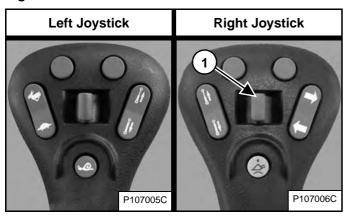
Move the Front Auxiliary Hydraulic switch (Item 1) [Figure 86] or [Figure 87] to the right or left to change direction of the auxiliary hydraulic fluid flow to the front quick couplers. If you move the switch halfway, the auxiliary functions move at approximately one-half speed. (EXAMPLE: Open and close grapple teeth.)
