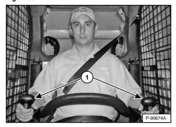
Both joysticks control drive and steering and are located on the left and right side in front of the seat (Item 1) [Figure 60].
