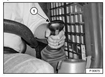
The joystick that controls drive and steering is on the left side in front of the seat (Item 1) [Figure 57].
