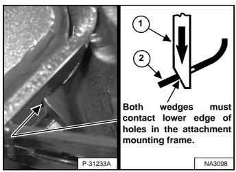
The wedges (Item 1) [Figure 308] must extend through the holes in the attachment mounting frame.
