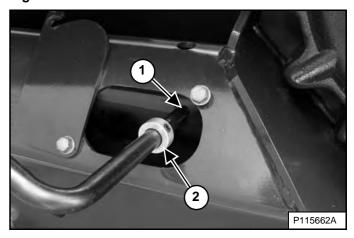
Install the bleed tool (7277225) on the track tension fitting (Item 1), adjust and tighten the collar (Item 2) **[Figure 263]** to fit behind the edge of the access cover.
