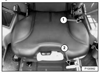
Pull the lever (Item 1) [Figure 106] up to adjust the angle of the seat back.
