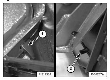
The wedges (Item 1) must extend through the holes (Item 2) **[Figure 138]** in the mounting frame of the bucket (or other attachment), securely fastening the bucket to the Bob-Tach.
