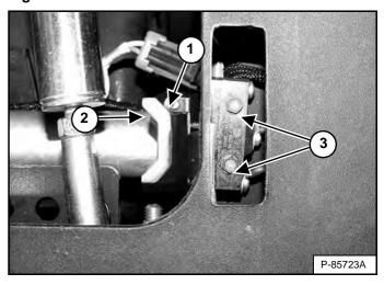
Loosen the screws (Item 3) **[Figure 177]** securing the back-up alarm switch. (Left side shown)
