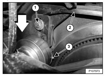
Push the spring loaded drive idler against the belt using a pry bar (Item 2). The pointer will be at the 90 degree position (Item 3) **[Figure 288]** when the idler is against the stop.
