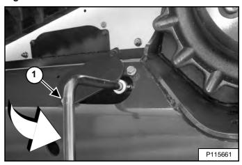
Tighten the access cover bolt (Item 1) [Figure 270] to secure the tool.
