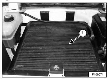
Use low air pressure or water pressure to clean the top of the hydraulic fluid cooler and radiator assembly (Item 1) [Figure 223].
