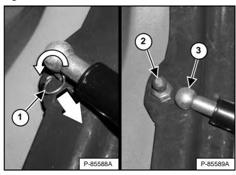
Rotate and pull the clip (Item 1) out of the gas spring socket. Pull the gas spring socket (Item 3) straight off the ball stud fitting (Item 2) [Figure 50].
