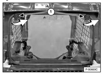
A kit is available to allow removal of the latch equipped rear window from outside the machine without tools. See your Bobcat dealer for availability.
