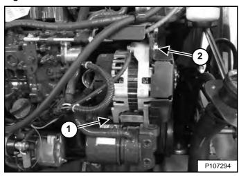
Loosen the bottom alternator mounting nut (Item 1) and loosen the top alternator adjusting bolt (Item 2) [Figure 277].
