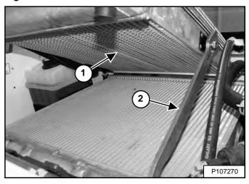
(Earlier Models with Square Coolant Tank) - Raise the hydraulic fluid cooler (Item 1) until the support bar (Item 2) [Figure 240] drops into position to support the hydraulic fluid cooler. This procedure will aid in draining the hydraulic fluid.
