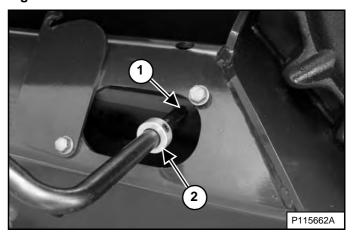
Install the bleed tool (7277225) on the track tension fitting (Item 1), adjust and tighten the collar (Item 2) **[Figure 272]** to fit behind the edge of the access cover.
