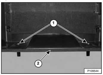
Clean the plenum drains (Item 1) [Figure 194] to ensure they are not plugged by debris.
