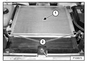
Use low air pressure or water pressure to clean the top of the air conditioning condenser (Item 1) [Figure 220].
