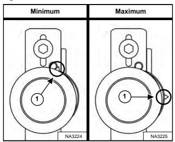
The pointer (Item 1) [Figure 283] on the spring loaded drive idler must be maintained between the two positions shown for correct belt tension.
