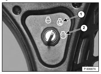
Turn the key switch to RUN (Item 1) [Figure 115]. The indicator lights on the left instrument panel will come ON briefly and the instrument panel / monitoring system will perform a self test.
