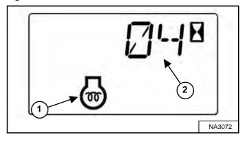
The machine will cycle the glow plugs automatically based on temperature. The engine preheat icon (Item 1) and the cycle time remaining (Item 2) [Figure 116] are displayed in the data display.
