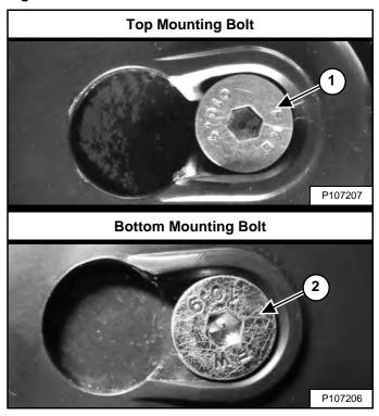
Position the drive belt shield over the drive belt shield mounting bolts. Slide the drive belt shield toward the front of the loader to fully seat the shield onto the top and bottom mounting bolts (Items 1 and 2) [Figure 289].
