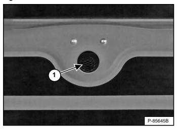
The back-up alarm (Item 1) [Figure 53] is located on the inside of the rear door.
