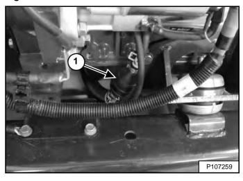
Squeeze the hand pump (priming bulb) (Item 1) [Figure 208] until fuel flows from the vent with no air bubbles.
