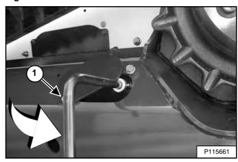
Tighten the access cover bolt (Item 1) [Figure 261] to secure the tool.
