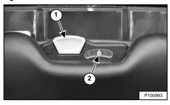
The lever (Item 1) is used to adjust the suspension response of the seat depending on the operator's weight. The optimum setting is achieved with the needle (Item 2) [Figure 109] centred in the gauge with the operator normally seated.
