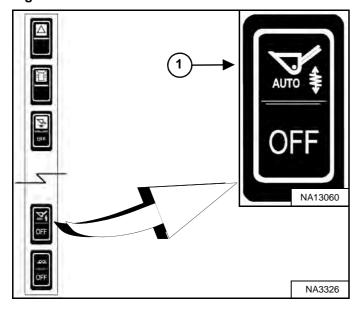
Press the top of the Automatic Ride Control switch (Item 1) **[Figure 83]** on the left switch panel to engage the automatic ride control function.
