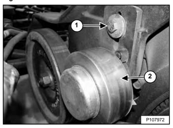
Loosen the spring loaded drive idler mounting bolt (Item 1) and allow the idler (Item 2) **[Figure 287]** to move up. Remove the mounting bolt, washer, and idler assembly.
