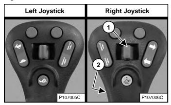
After activating the auxiliary hydraulics, press the Continuous Flow Control switch (Item 2) [Figure 88] or [Figure 89] to allow constant auxiliary hydraulic fluid flow to the front female coupler (female coupler is pressurised). (EXAMPLE: Operate a backhoe.)
