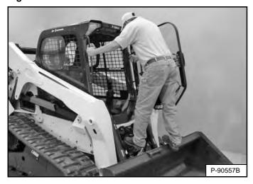
Use the bucket or attachment steps, grab handles, and safety treads (on the loader lift arms and frame) to get on and off the loader, maintaining a three-point contact at all times [Figure 104]. Do not jump.
