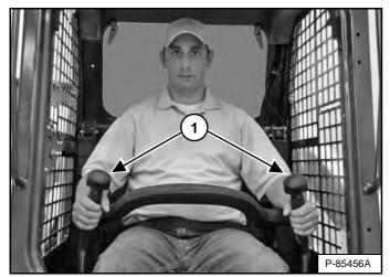
The steering levers (Item 1) [Figure 54] are on the left and right side in front of the seat.
