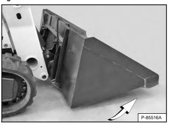
Tilt the Bob-Tach backward until the cutting edge of the bucket (or other attachment) is slightly off the ground [Figure 136]. This procedure will cause the bucket mounting frame to fit up against the front of the Bob-Tach.
