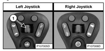
Move the Rear Auxiliary Hydraulic switch (Item 1) **[Figure 97]** or **[Figure 98]** to the left and right several times. Turn the key switch to STOP.
