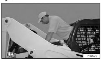
Exit through the rear of the operator cab [Figure 42].
