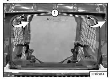
The rear window can be removed from outside the loader using a T40 TORX® Drive tool. Turn both screws (Item 1) [Figure 45] anticlockwise until the latches disengage from the window frame. Pull the top of the window away from the cab and lift up to remove.
