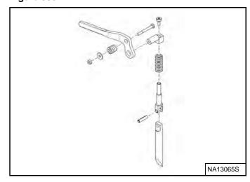
Inspect the mounting frame on the attachment and Bob-Tach, linkages, and wedges for excessive wear or damage [Figure 306]. Replace any parts that are damaged, bent, or missing. Keep all fasteners tight.
