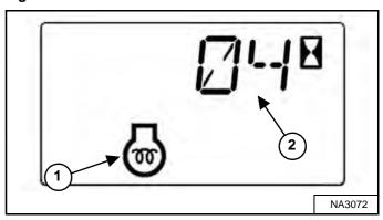
The machine will cycle the glow plugs automatically based on temperature. The engine preheat icon (Item 1) and the cycle time remaining (Item 2) [Figure 121] are displayed in the data display.
