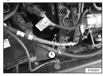
Install the drive belt shield bolt (Item 1) [Figure 290].
