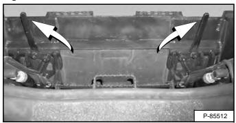
Pull the Bob-Tach levers up [Figure 139] until they are fully raised (wedges fully raised).
