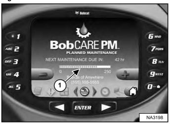
The Deluxe Instrumentation Panel (if equipped) will display a bar (Item 1) [Figure 316] showing the time remaining until next service. This bar will turn red when service is past due. [NEXT MAINTENANCE DUE] will change to [MAINTENANCE PAST DUE] and display the number of hours past due.
