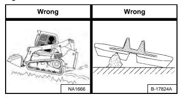
Avoid operating or turning on sharp objects such as jagged rocks, broken concrete, quarry materials, or scrap applications. This can cause cuts on the lug surface of the tracks [Figure 154].
