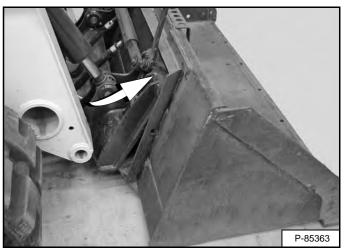
Drive the loader slowly forward until the top edge of the Bob-Tach is completely under the top flange of the bucket mounting frame [Figure 143] (or other attachment).
