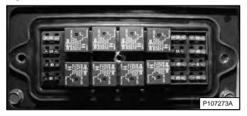
Remove the fuse panel cover to check or replace the fuses and relays [Figure 230].
