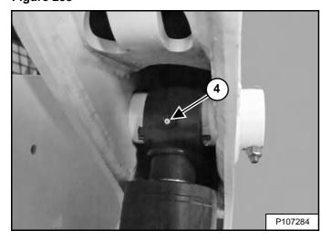
4. Rod End Lift Cylinder (Both Sides) (2) [Figure 295].
