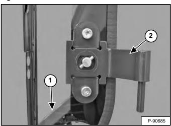
Orient the latches as shown (Item 1) and install the door hinges (Item 2) **[Figure 51]** on the door. (Bottom hinge shown.)
