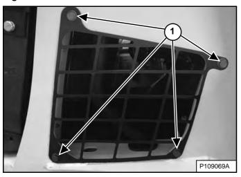
Remove the left side access cover bolts (Item 1) **[Figure 246]** and remove the access cover. (Lift arms shown raised for visual clarity.)
