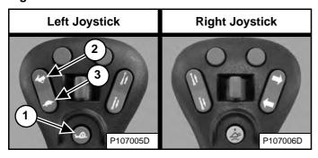
Adjust the speed percentage higher (Item 2) or lower (Item 3) **[Figure 67]** by pressing the Speed Control switch until the desired default setting is displayed.
