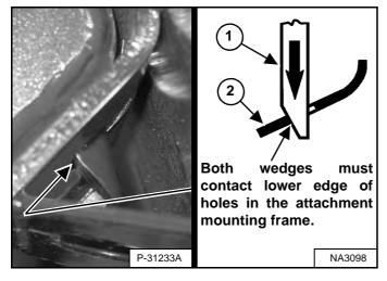
The wedges (Item 1) [Figure 305] must extend through the holes in the attachment mounting frame.
