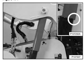
Lower the lift arms slowly until the lift arm support device is held between the lift arms and the lift cylinder. The tabs of the lift arm support device must go past the end of the cylinder (Inset) [Figure 171].
