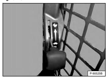
Set the engine speed control to the low idle position [Figure 119].
