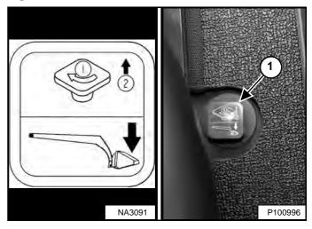
The lift arm bypass control (Item 1) **[Figure 39]**, located to the right of the operator's seat, is used to lower the lift arms if the lift arms cannot be lowered during normal operations.
