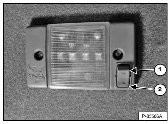
Push this side of the switch (Item 1) to turn the light ON. Push this side of the switch (Item 2) **[Figure 30]** to turn the light OFF.
