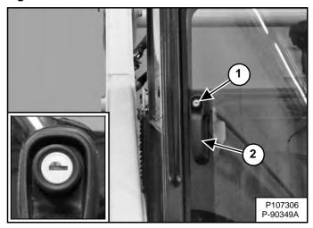
Push the knob (Item 1) and pull the handle (Item 2) to open the front door. A lock is provided in the knob (Inset) [Figure 26] to lock the front door when the loader is not in use.
