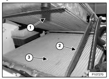
Raise the hydraulic fluid cooler (Item 1) until the support bar (Item 2) drops into position to support the hydraulic fluid cooler. Use low air pressure or water pressure to clean the top of the radiator (Item 3) [Figure 219].
