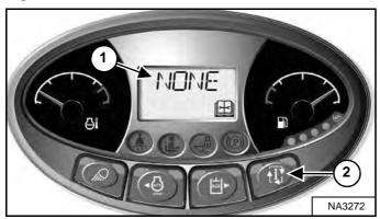
Press the Information button (Item 2) to cycle the data display (Item 1) **[Figure 310]** until the service code screen is displayed. If more than one service code is present, the codes will scroll on the data display.
