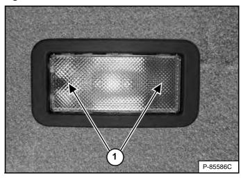
Push either side of the lens (Item 1) [Figure 31] to turn the light ON. Return the lens to the middle position to turn the light OFF.
