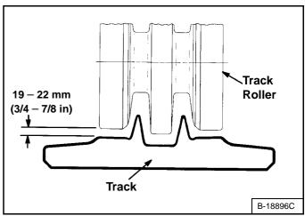
DO NOT put your fingers into the pinch points between the track and the roller. Use a 19 - 22 mm (3/4 - 7/8 in) bolt, dowel or block to check the gap [Figure 257] and [Figure 258].
