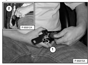
NOTE: The 3-point restraint must be used when selecting high range operation [Figure 62].
