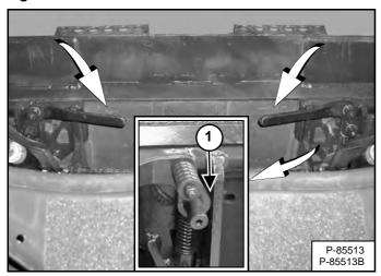
Push down on the Bob-Tach levers until they are fully engaged in the locked position [Figure 137] (wedges fully extended through the attachment mounting frame holes).
