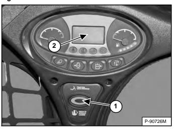
Press the PRESS TO OPERATE LOADER button (Item 1) **[Figure 118]** to activate the BICS<sup>™</sup> and to perform hydraulic and loader functions.
