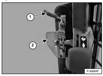
Pull the front door closed using the handle (Item 2) [Figure 27].
