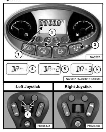
Press the Information button (Item 3) to cycle the data display until the drive response menu is displayed. The current drive response setting will appear in the data display (Item 1) [Figure 69].
