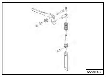
Inspect the mounting frame on the attachment and Bob-Tach, linkages, and wedges for excessive wear or damage **[Figure 309]**. Replace any parts that are damaged, bent, or missing. Keep all fasteners tight.
