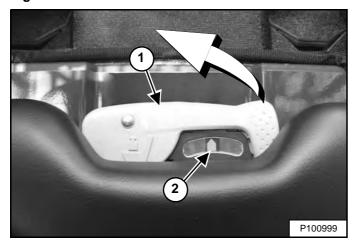
The lever (Item 1) is used to adjust the suspension response of the seat depending on the operator's weight. The optimum setting is achieved with the needle (Item 2) [Figure 107] centred in the gauge with the operator normally seated.
