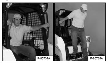
Exit the loader using grab handles, safety tread, and steps (maintaining a three-point contact) [Figure 132].
