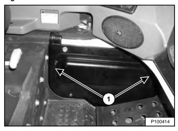
The fuse / relay panel is located behind an access panel near the left foot pedal / footrest. Pull the panel at each end (Item 1) [Figure 228] to remove.
