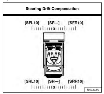
Steering drift compensation contains a total of 21 settings. Steering drift compensation can be set to any point from NEUTRAL to [SFL10] or [SRL10] left, and from NEUTRAL to [SFR10] or [SRR10] right. [SF---] or [SR---] is displayed when set for NEUTRAL [Figure 70].
