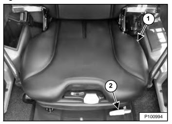
Pull the lever (Item 1) [Figure 108] up to adjust the angle of the seat back.
