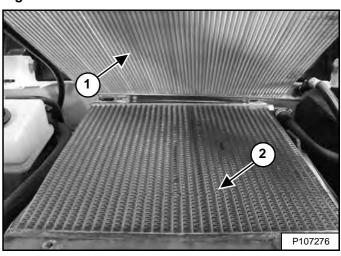
NOTE: Be careful when raising and lowering the air conditioning condenser so that the air conditioning condenser does not fall on the hydraulic fluid cooler and damage the fins.
