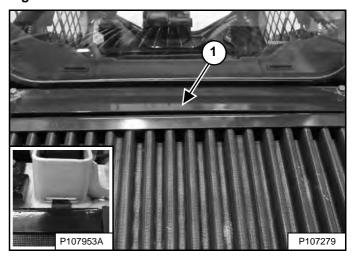
Align the edge of the rear grille under the shield (Item 1), insert the tabs into the slots (Right Side Shown) (Inset) [Figure 189], and lower.
