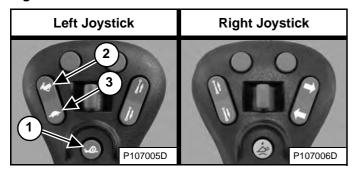
Press the button (Item 1) [Figure 65] on the left joystick once to engage Speed Management.
