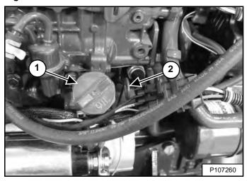
Park the loader on a level surface. Stop the engine. Open the rear door and remove the dipstick (Item 2) [Figure 209].
