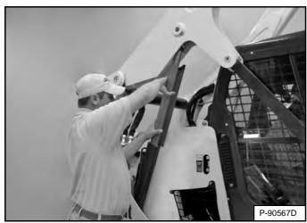
Have a second person remove the lift arm support device [Figure 172].
