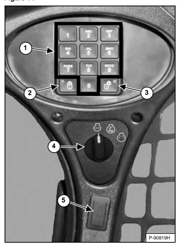
This machine may be equipped with a Keyless Start Panel [Figure 14].
