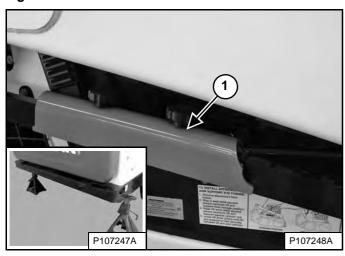
Put jackstands under the rear corners of the loader frame (Inset) [Figure 169].
