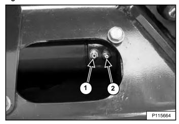
Loosen the access cover bolts and pivot the access cover open [Figure 259].
