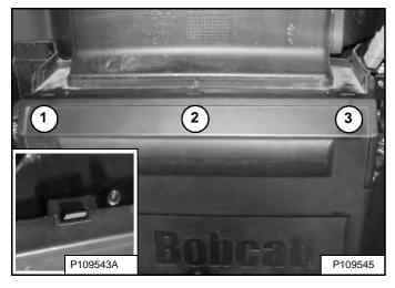
2. Push the cover up in three places (Items 1, 2, and 3) until the slots snap into place on the tabs. This slot (Inset) [Figure 197] is correctly fastened.
