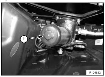
Put a suitable container below the filter housing and remove the filter housing (Item 1) [Figure 248].
