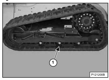
Raise one side of the loader and put jackstands at the front and rear of the loader frame so that the track is about 76 mm (3 in) off the ground [Figure 265]. Lower the loader to the jackstands. Be sure the jackstands do not touch the tracks.
