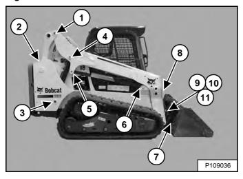
The grease fitting locations [Figure 291] are shown in more detail in the following figures.
