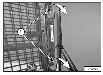
Turn both latches (Item 1) [Figure 48] down until they disengage from the door frame.
