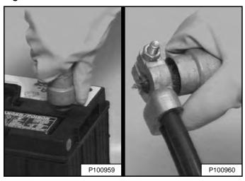
The battery cables must be clean [Figure 232] and tight.
