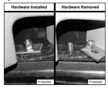
Remove the nuts and washers [Figure 181] (both sides) at the front corners of the operator cab.
