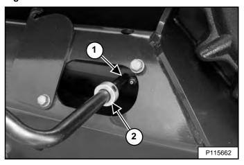
Install the bleed tool (6675936) on the bleed fitting (Item 1), adjust and tighten the collar (Item 2) [Figure 260] to fit behind the edge of the access cover.
